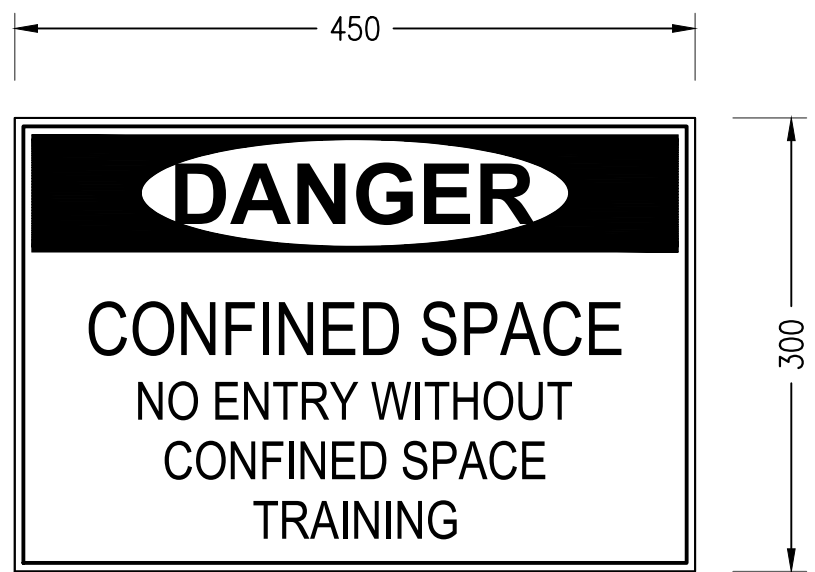
CONFINED SPACE SIGN DETAIL SCALE 1:20
